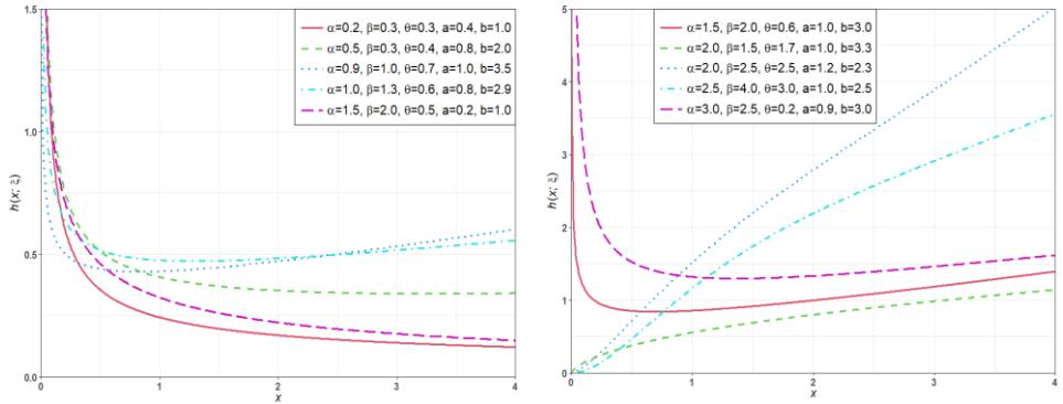
Figure 6: Hazard Rate Plots of the GLFR-Lx Distribution for Some Parametric Values
