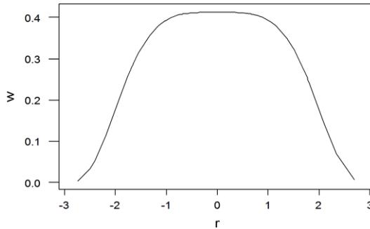
**Figure 4: Graph of weight function of the new Redescending M-estimator**
